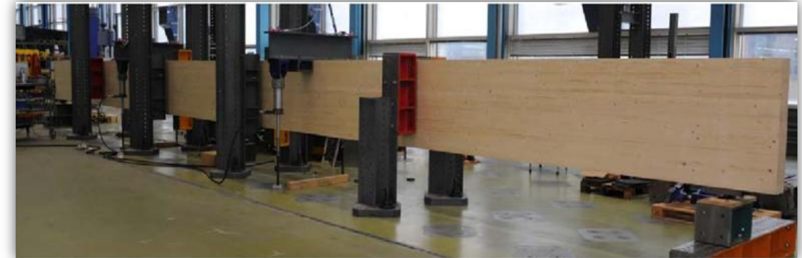
Full scale four point bending test
