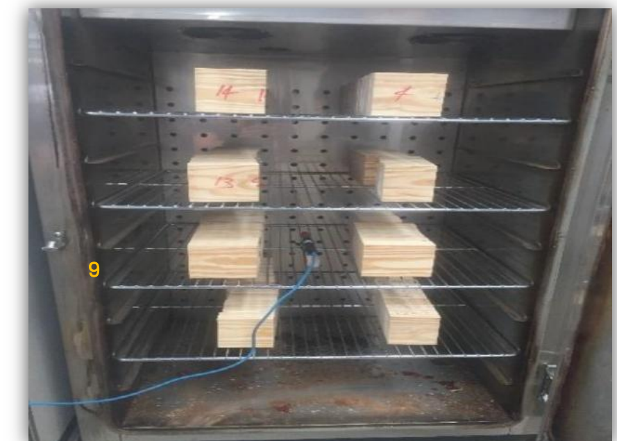
Samples in hot air oven for delamination
