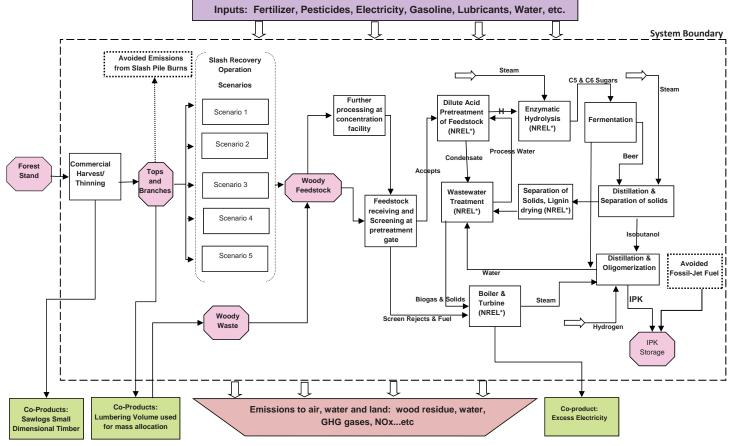
Figure 1: Overall scope for LCA of the woody biomass to bio-jet fuel process.
