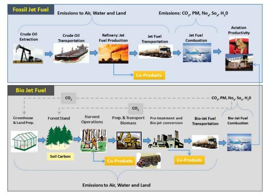
Figure 5. Comparing the LCA's of fossil based jet fuel against bio-jet fuel
